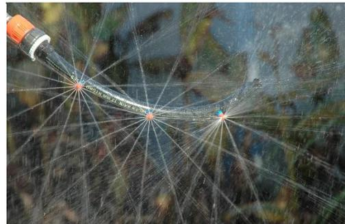
MicroJetSprayers were used due to their strong and functional spray pattern to different angles and their compact design.
