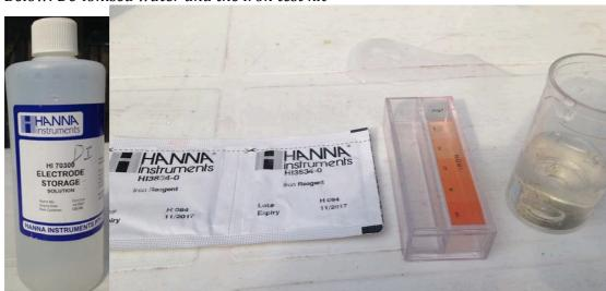
Nitrate was measured using a nitrate photometer, that utilised a cadium reaction method. The photometer required a sample of water to be inserted in the photometer's cuvette.
