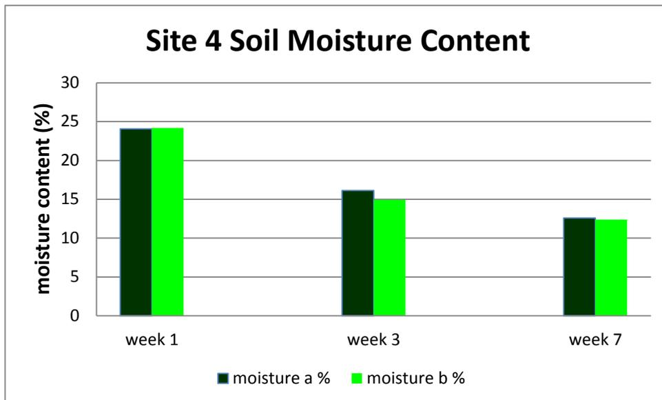
Figure 7. compares the moisture content of the soils in Site 4. Measurements shown are the moisture percentage of soil dry weight.
