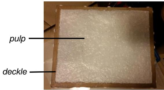
*Fig. 4 – pulp formed a sheet of paper across the screen*
