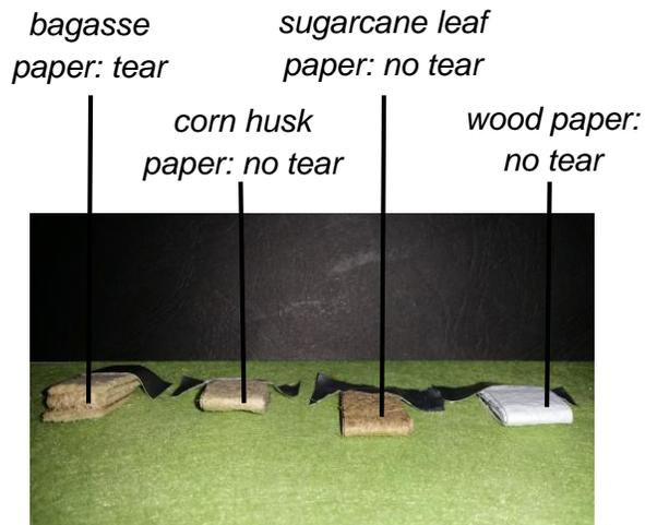
Fig. 10 – samples of all four types of paper on fold 2
