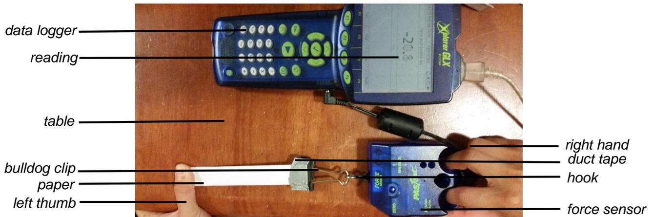
*Fig. 7 – Tensile Strength Test Setup*
