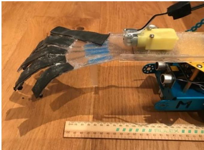
**Figure 6** Measuring when Ultrasonic sensor should trigger gripping
