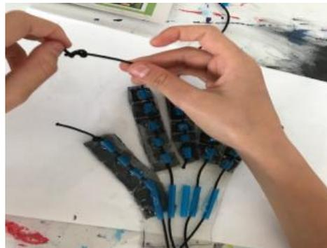
Figure 9 Assembled fingers with straws and strings
