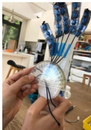
Figure 5 Measured degrees needed for motor to fully close grip
