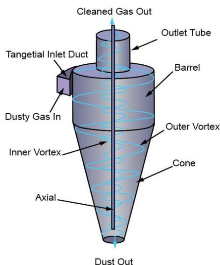
As the substance rotates in this spiral, particles in it are thrown against the outer wall. While substances are forced to change direction as they rotate, the inertia of heavier particles force them to continue in their original direction (that of their tangential entry). In this way, particles become separated.
