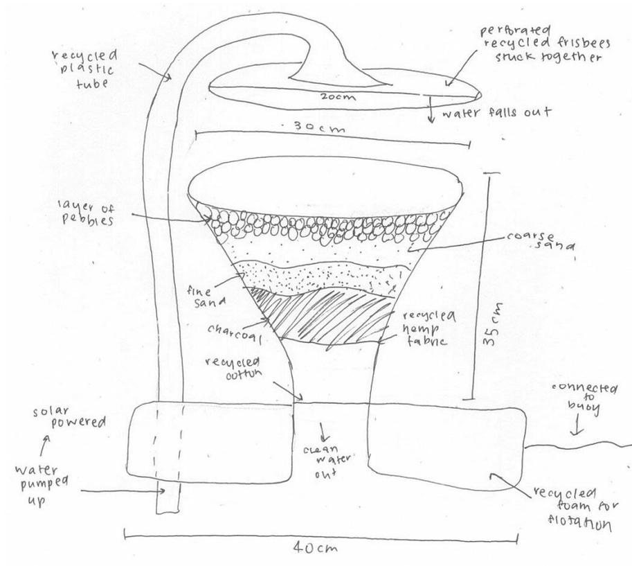
Concept 1 was chosen as its use hydrocyclonic technology, but was changed to stand vertically and to have a conical collection chamber similar to existing cyclones and so making it more likely to work. A buoy was added, to give the separator buoyancy and to protect electrical parts.
