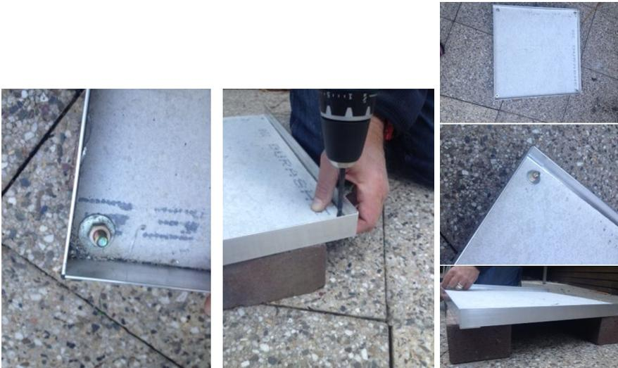
10. I laid the 3 felt layers over the panel, and, using the fabric scissors, made an incision where I poked through the bolt. I then fastened the nut and the locking nut to keep them in place.
